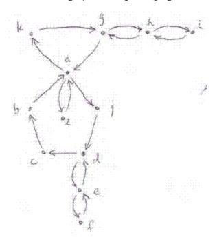
isolate the nodes making up the pentagonal cycle (a, b, c, d, and j) and form a partitioned matrix
