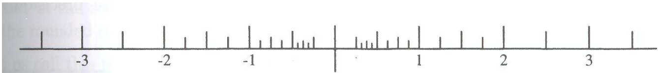
Figure 2.3: Machine numbers on a toy binary computer
