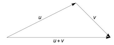
• Draw vectors  $\vec{u}$  and  $\vec{v}$  with initial points together. The two vectors form two sides of a parallelogram. Complete the parallelogram. Draw the vector sum from the initial points of  $\vec{u}$  and  $\vec{v}$  to the opposing vertex of the parallelogram.
