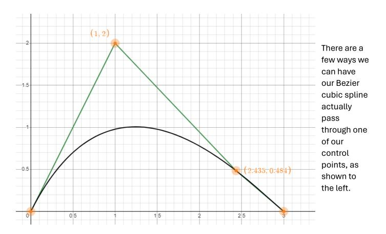
The only way for our Bezier cubic spline will run through both control points  $P_1$  and  $P_2$  is if all four control points fit linearly.
