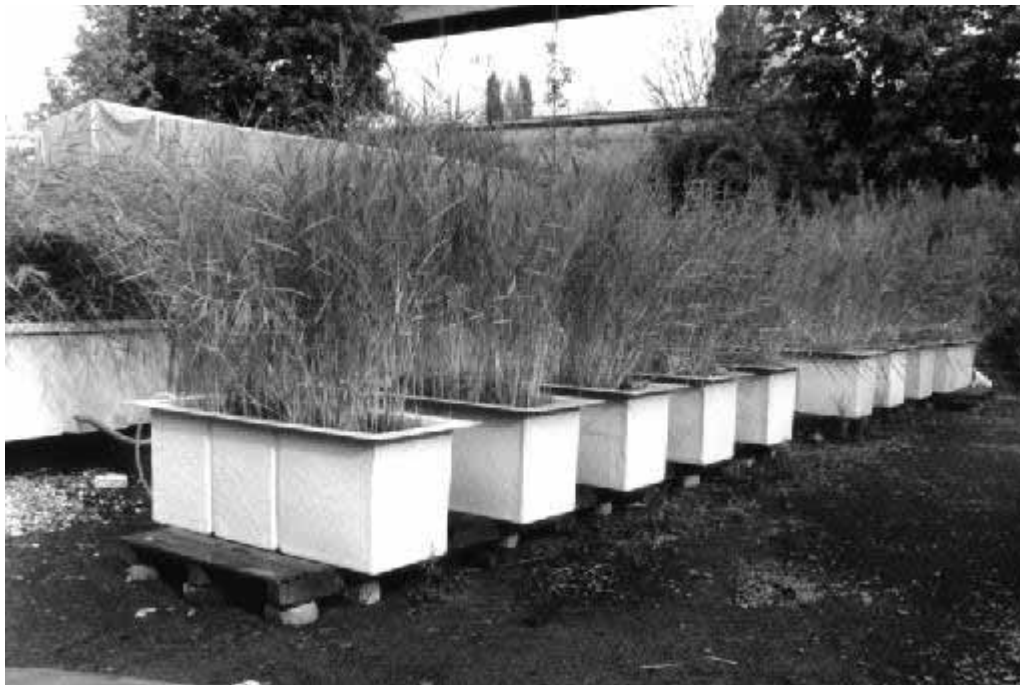
Figure 4: Tests with mobile pilot plants support the choice of filler material and reed strain for application in special cases.
